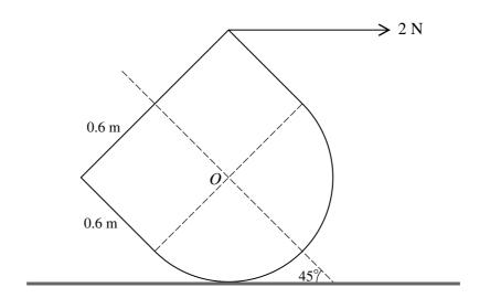
The solid is placed with the curved surface of the hemisphere on a rough horizontal surface and the axis inclined at  $45^{\circ}$  to the horizontal. The equilibrium of the solid is maintained by a horizontal force of 2N applied to the highest point on the circumference of its plane face (see diagram). Calculate
